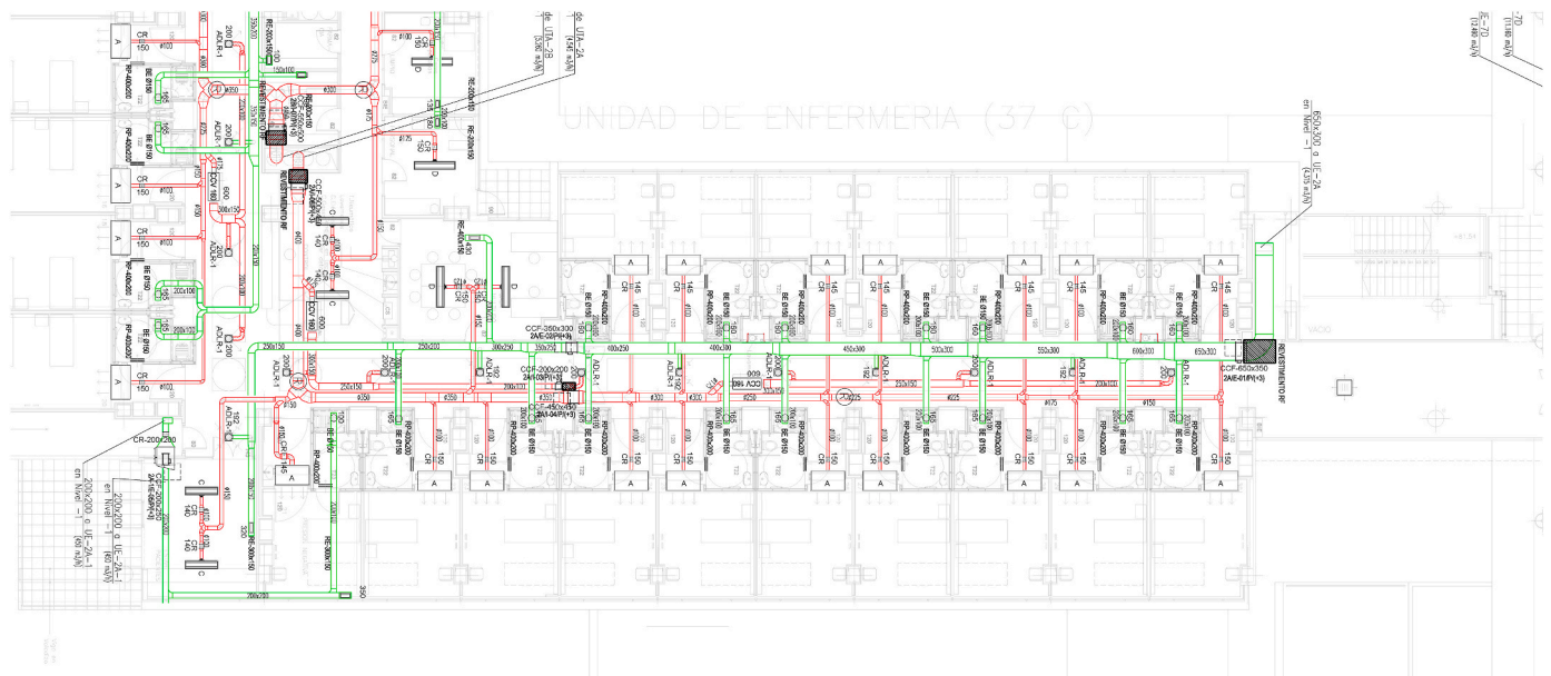
Fig. 3. Detailed description of the ventilation system in the Covid-19 and non-Covid-19 areas of Fig. 1. The green and red lines indicate the air inlet and outlet pipes. (For interpretation of the references to colour in this figure legend, the reader is referred to the Web version of this article.)
